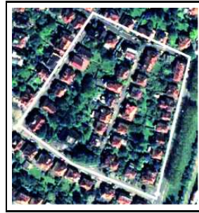
(b) Aggregate object composed of some groups of homogeneous pixels (houses, gardens, road).
