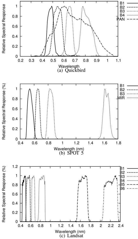
Fig. 1. Example of three *Relative Spectral Response* (RSR).
