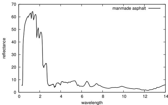
Fig. 3. Example of a full spectrum of a man-made asphalt extracted from the ASTER library.
