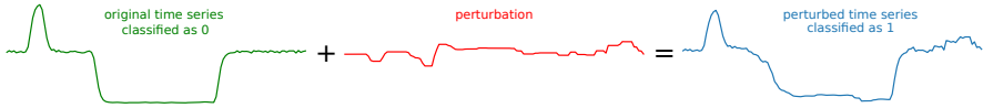
Fig. 1: Scheme of adversarial attack. Time series from the BME dataset, perturbation generated with SGM, not represented at scale.
